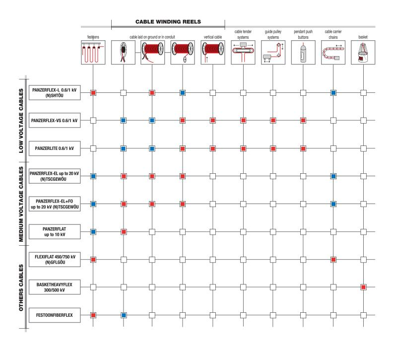
The above table is designed in order to give an easy reference in cable selection for the main mobile equipment application. Please keep in mind that when using this guide all the concurrent factors are to be considered: bending radii, speed, ambient temperature and tension. Even if only one of these parameters stands outside the given data of this catalogue, please contact our sales department for gaining further information.
